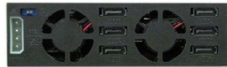
Dual 40mm Fans / Molex Power 6 Channel SATA Port
