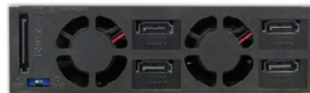
Dual 40mm Fans / SATA Power 4-channel SATA Port
