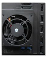
7pin Data x5 and 15pin Power x2 Connector
